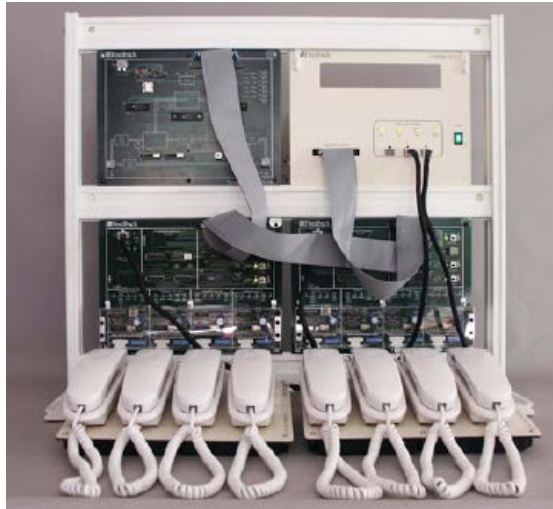
Fig. 4. The whole Digital Switching system.
